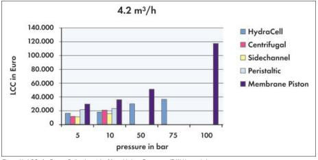
Figure 2b: LCCs for Pumps Delivering 4.2 m<sup>3</sup>/hr at Various Pressures. (F-W Hennecke)
