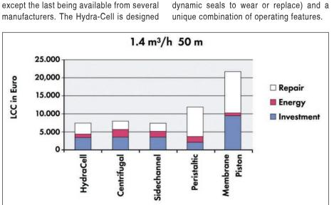
Figure 2a: LCCs for Pumps Delivering 1.4 m³/hr at 5 bar. (F-W Hennecke)
